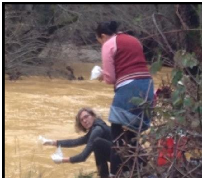
TSF Staff Alex Keeble Toll M.A., M.Sc., and Carrie Monohan Ph.D. sample the turbid water in Deer Creek in Nevada City, during a typical storm when the creek ran orange, a color associated with discharge from hydraulic mine landscapes.
