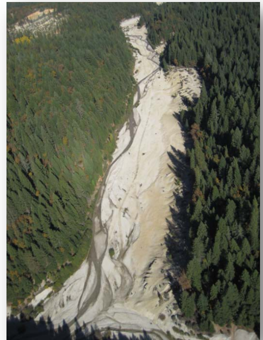
Figure 1: Greenhorn Creek, a tributary to Rollins Reservoir - Photo taken in 2010 shows the creek channel still choked with hydraulic mining debris. (Photo: Nevada Irrigation District)
